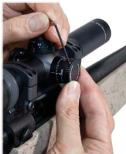
Align the windage turret cap.
